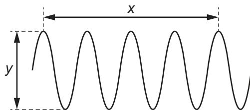
Which row gives the wavelength and the amplitude of the wave?
